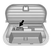
This vehicle may have a tire sealant and compressor kit in place of a jack or spare tire. It is located in a foam container in the rear compartment storage area. If the vehicle has a cargo cover, see *Cargo Management System on page 4-5* for instructions on how to access the tire sealant and compressor kit.
